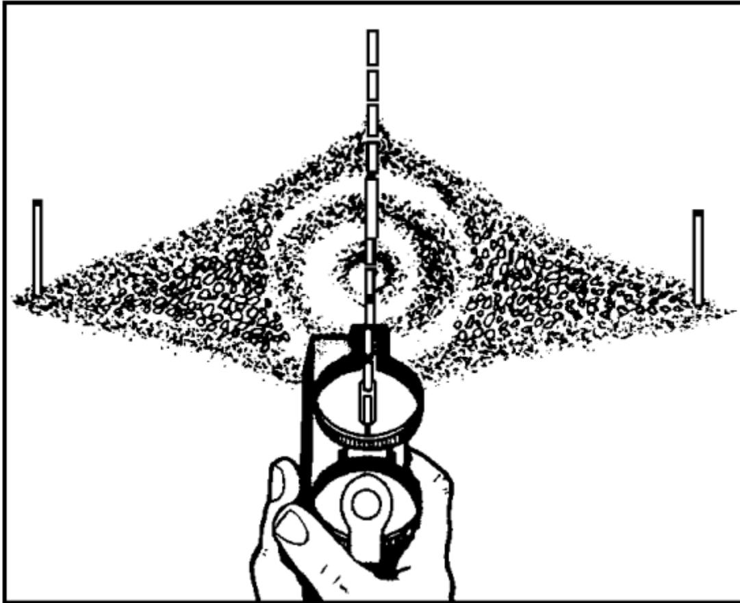
Figure 1-6. Measuring direction - side spray method.
