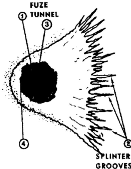
Figure 1-9. High-angle mortar crater.
