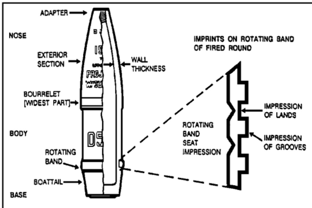
Figure 1-13. Typical shell, showing critical measurements.
