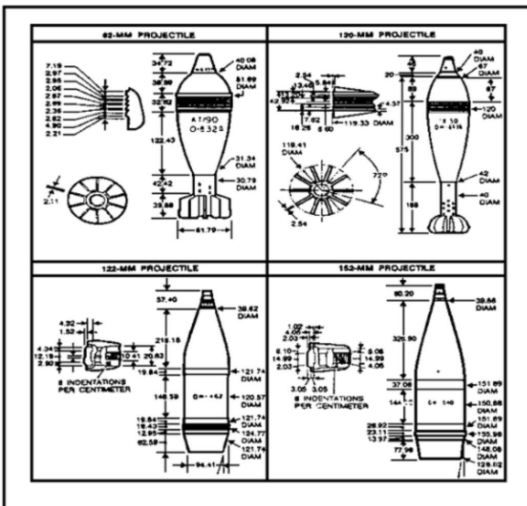
Figure 1-15. Some standard Soviet artillery and mortar rounds.
