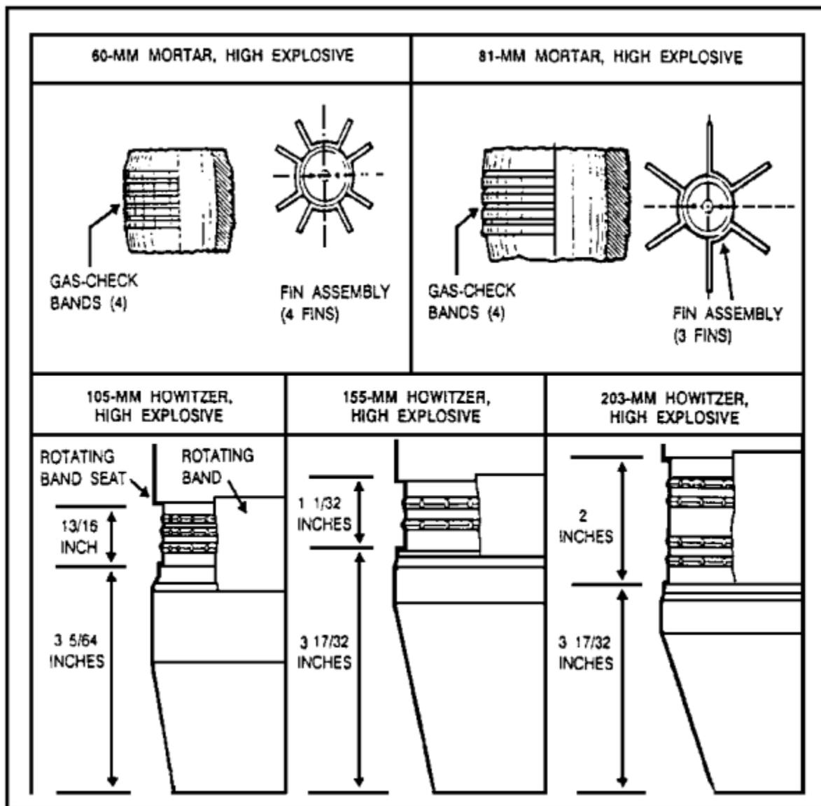
Figure 1-16. Shell fragment and tailfin identification, US ammunition.
